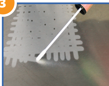
Grasping black housing pull away from orange swab housing to expose the premoistened swab. Swab an area 100 cm 2 (16 in 2 ). Rotate the handle to achieve full swab contact with surface
