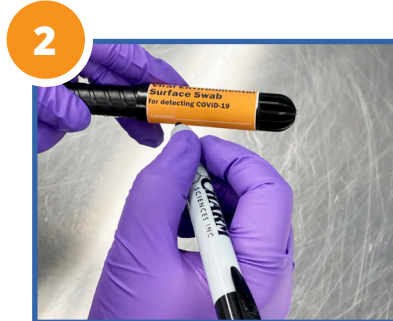
Identify the sample. The device features a write-on-label to document swab location, date, and time
