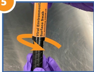
5 Reinsert the swab into the cartridge housing by turning clockwise so that it is airtight
