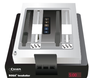
For batch processing, incubate multiple strips simultaneously, then read results in the Charm EZ system.
