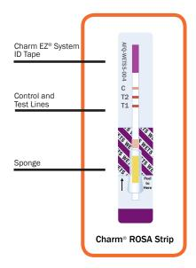
The ROSA® WET®-S5 Aflatoxin Quantitative Test (AFQ-WETS5) delivers rapid and accurate results using ROSA (Rapid One Step Assay) lateral flow technology. Water Extraction Technology eliminates ethanol and methanol using an extraction powder and water (e.g., bottled) to quickly and safely extract aflatoxin from the sample.
