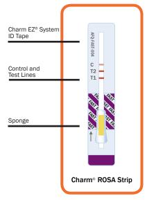
The **ROSA® FAST Aflatoxin Quantitative Test (AFQ-FAST)** delivers rapid and accurate results using ROSA (Rapid One Step Assay) lateral flow technology. ROSA mycotoxin tests are simple to run; just add the diluted sample extract to the strip, incubate for 3 or 5 minutes, and read results in the Charm EZ-M system.
