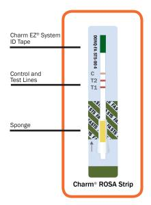
The ROSA® FAST5 DON Quantitative Test (DONQ-FAST5) delivers rapid and accurate results using ROSA (Rapid One Step Assay) lateral flow technology. The diluted extract is applied to the test strip, incubated for 5 minutes, and read in the Charm EZ-M system.
