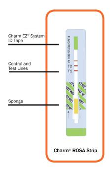
The ROSA® WET®-S5 Fumonisin Quantitative Test (FUMQ-WETS5) delivers rapid and accurate results using ROSA (Rapid One Step Assay) lateral flow technology. Water Extraction Technology eliminates ethanol and methanol using an extraction powder and water (e.g. bottled) to quickly and safely extract fumonisin from the sample.
