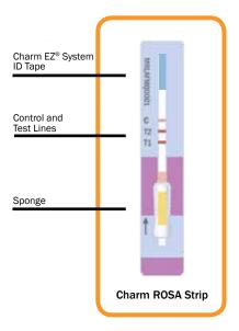
The Charm® MRL Aflatoxin M1 Quantitative Test delivers rapid and accurate results using ROSA<sup>®</sup> (Rapid One Step Assay) lateral flow technology. The MRLAFMO is the only quantitative lateral flow test that detects aflatoxin M1 in milk at the EU MRL of 0.050 ppb (50 ppt).
