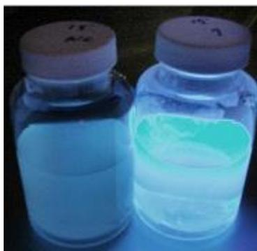
←Figure 3. UV 366 nm light image of negative and positive test.
